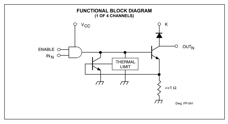
NOTE: These devices do not include an absolute thermal shutdown. Package power dissipation under fault conditions (2.4 W in the faulted channel) must therefore be evaluated at maximum operating temperature.
